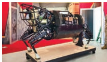
The Marine Corps Warfighting Lab is experimenting with the legged squad support system, an autonomous robot intended to help reduce the loads that Marines carry.
