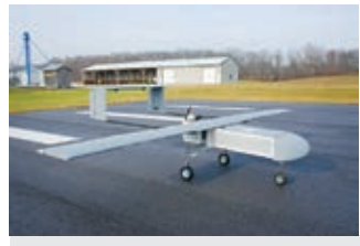
The SPAARO Unmanned Aerial System, developed to carry a 10-pound payload for more than one hour. The VaCAS fleet sports more than a dozen types of fixed and rotary wing unmanned aircraft.
